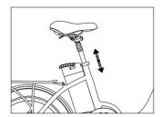
To enable comfortable, fatigue-free and safe riding, the saddle height should be adjusted to the body size of the rider.
