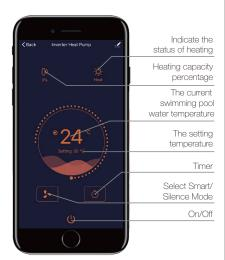
2. For heat pump with Heating & Cooling function:
